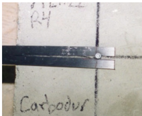
Figure 2.1 – Splitting Failure for existing FRP Laminates (Lamanna 2002)
