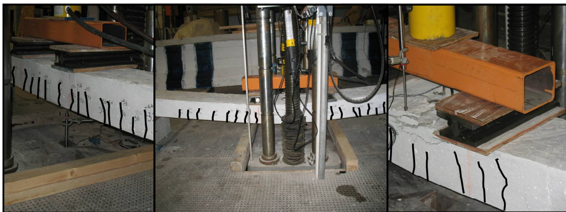
Figure 4.1 – Crack pattern and failure: control specimen
