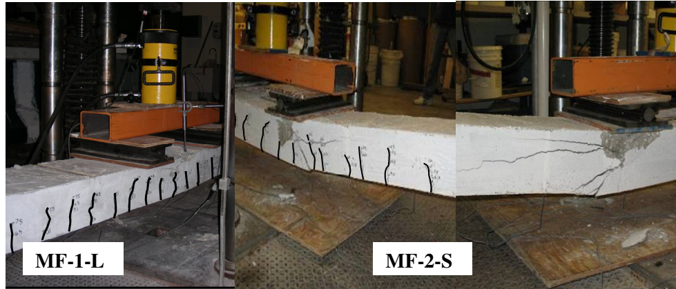
Figure 4.4 – Crushing of the concrete in the slabs MF-1-L and MF-2-S
